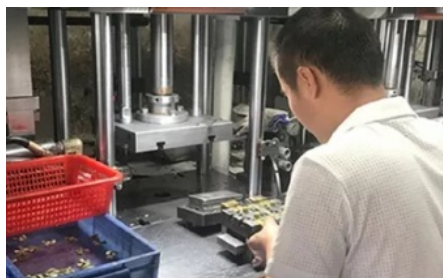
Injection of wax mold
