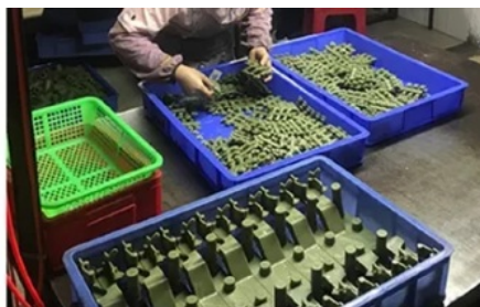
Repair wax mold
