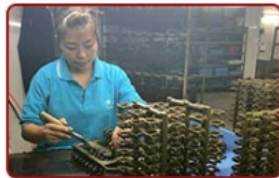
4 Group Wax Mould To Tree
